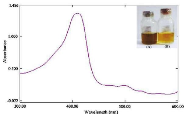
**Fig. 2.** UV-visible range spectra of AgCl-NPs synthesized by *Anabaena variabilis* ethanol extract. Visual changes in colour of silver nitrate solution  $10^{-3}$  M; (A) represents the developed colour after adding *A. variabilis* ethanol extract with brown colour and (B) represents the original colour of algal extract (control).
