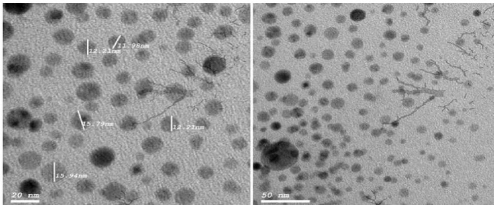
**Fig.3.** Representative TEM micrograph of AgCl-NPs synthesized by the reduction of  $10^{-3}$  M  $\text{Ag}^+$  ions by the ethanol extract of *Anabaena variabilis*.
