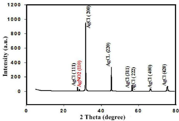
**Fig.5.** XRD pattern of AgCl-NPs synthesized by reduction of  $10^{-3}$  M  $\text{Ag}^+$  ions by the ethanol extract of *Anabaena variabilis*.
